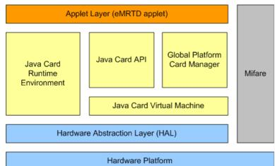
• The MRTD's chip circuitry and the IC dedicated software forming the Smart Card Platform (Hardware Platform and Hardware Abstraction Layer);
